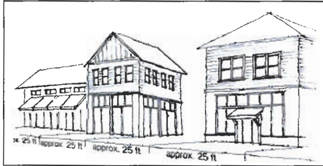
▲ The sketch above shows how design elements can be applied to create a "storefront appearance".
