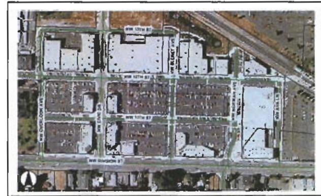
▲ This aerial view of Gresham Station (Gresham, OR) shows how the buildings have been sited to break up large parking areas and provide "internal streets" that contribute to a high-quality pedestrian environment
